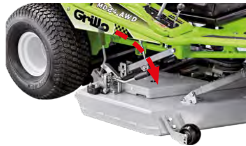
Rear discharge cut Open cutting chamber Mulching cut Closed cutting chamber
